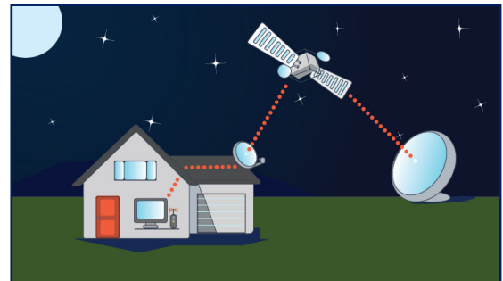
Figure 1: Explaining satellite connectivity. Source: https://www.reviews.org/internet-service/satellite-internet-work/
