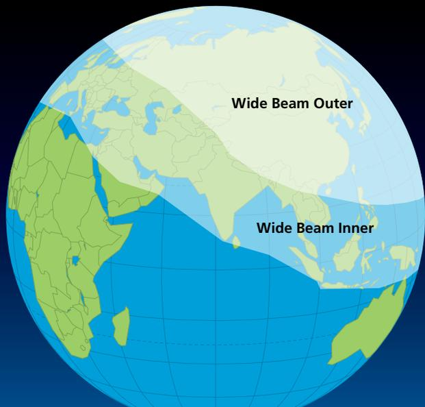
Fig. 2: IS-33e Ku-band Wide Beam
