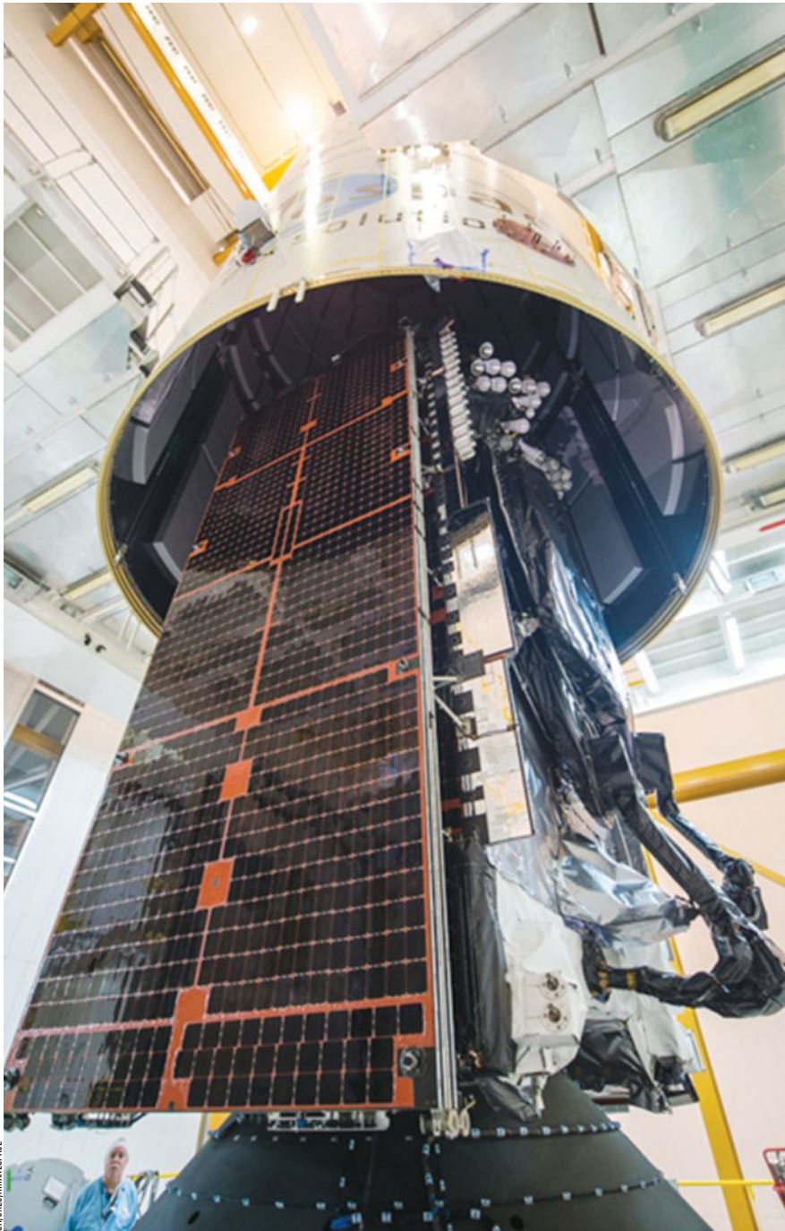
▲ The Intelsat 29e in the Final Assembly Building being loaded onto the top of the Ariane 5 second stage.
